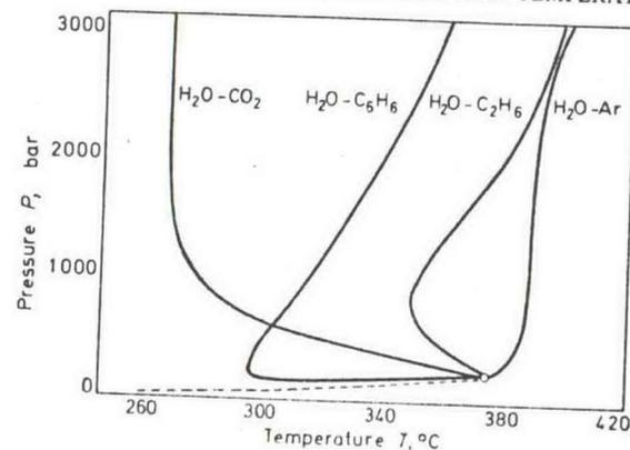
Figure 12. Critical curves of several binary aqueous systems.
